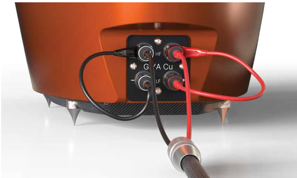
Fig 3. For many folks the use of extra wires will seem quite pointless in which case a single pair of good quality conductors will be all you require and the two pairs of terminals must be linked at the speaker using the links provided. In the accessories pack you will find two 10cm lengths each of red and black wire each terminated with a 4mm plug and spade. Link the hi-mid section to the low section as shown in Fig.3. supplied non bi-wired links.
